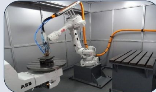
Robotic Laser Cladding Machine for Valve Seat
